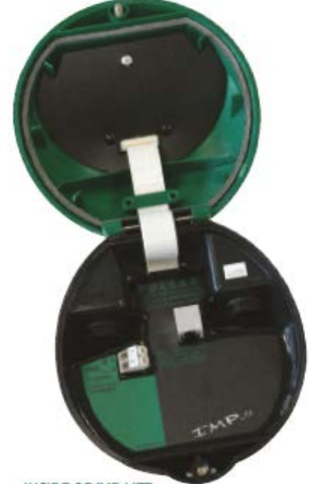
INSIDE OF IMP LITE SHOWING RJ11 PORT
