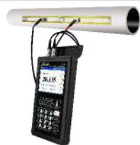
Transmitter and Transducer
