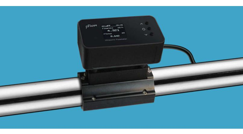
Clamp-on type ultrasonic flow meter is for the difficulty of installing a conventional model in an old building. It features with clamp-on measurement, no need to cut pipes and to shut down machines. Easy operation menu Displaying Instantaneous Flow and Selecting Flow Units Optional unit, m3/h, I/m, gpm(UK), cfm, gpm(USA)
